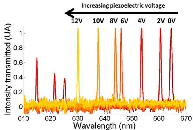
Fig. 1 Filter transmission showing wide range single mode tunability. The transmission lines indicated are  $\text{TEM}_{00}$  modes (see text). The weaker transmission lines below 625 nm are  $\text{TEM}_{01}$  modes.
